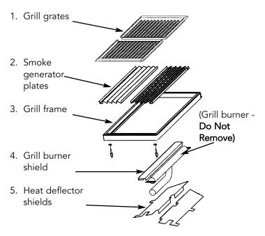
Clean greasy parts with a household grease solvent such as household ammonia and water. If necessary, a soap filled steel wool pad can be used on the grill frame shield, grill burner, and grill heat deflector.
